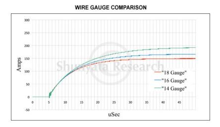
Wire Gauge Comparison: This graph plots the differences between power cables of different wire gauge size. These measurements were generated by the DTCD® Analyzer from actual stock power cords. Notice the progressive improvement in instantaneous power delivery as the wire gauge is increased from 18 to 16 to 14 gauge\*. \*(Wire gauge is inversely proportional to the number - 18 is smallest and 14 is largest).
