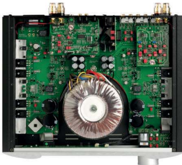
Inside the Neo 340i: Note the four bipolar output transistors each side.
