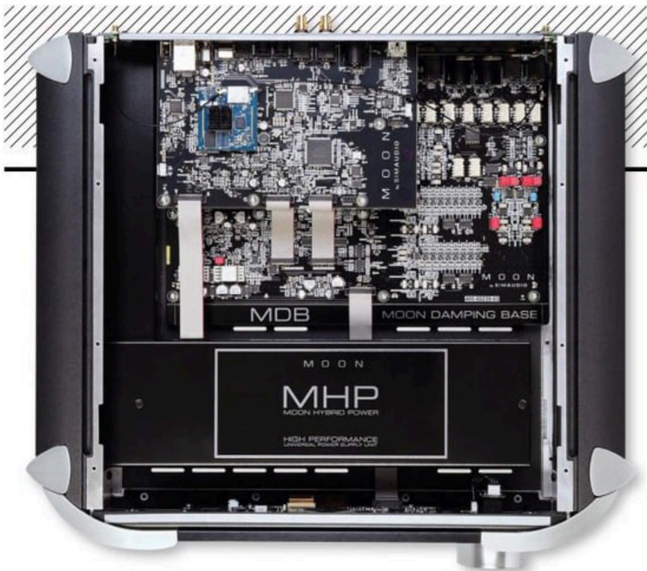
ABOVE: Switchmode MHP PSU has separate supplies for the digital board [top left] with its StreamUnlimited Wi-Fi/streaming platform, XMOS USB microcontroller and AK4137EQ SRC. Two ES9038PRO DACs are on the (compliantly mounted) main PCB [underneath] with an ES9822QPRO ADC [centre], line and phono stages [top right]
