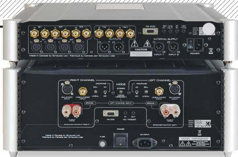
ABOVE: The preamp [top] offers five line ins (3x RCAs, 2x XLRs), three line outs (2x RCAs and 1x XLR). Outboard PSU inputs are also included. The power amp [below] has balanced (XLR) and single-ended (RCA) ins, AC/DC coupling and bridged modes
