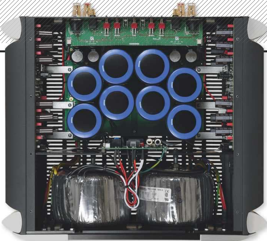
ABOVE: Constructed as a dual-mono (and bridgeable) amplifier, much of the 860A v2's 40kg weight is accounted for by the two huge toroidal mains transformers [bottom] feeding 2x120,000µF of reservoir capacitance [blue]. The output devices are mounted on concealed heatsinks [left and right]
