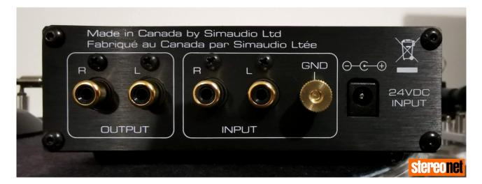
Around the rear, you'll find two output and two input RCA jacks, and a ground post, all of which are goldplated. There's also the input jack for the 24V power supply which remains on at all times. Don't worry though; this thing sips at the juice. Even the wall wart power supply looks better than average with its fabric-covered cord. After plugging everything in and setting the switches to where they needed to be it was time to get going.
