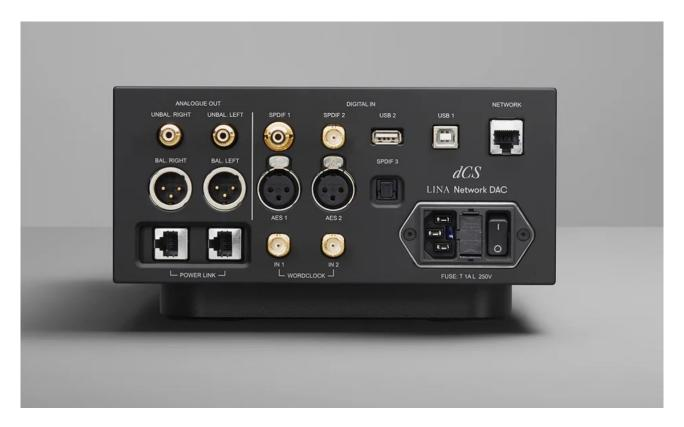
The converter within the LINA is the Ring DAC that first saw consumer audio use in the Elgar in 1996. The technology was first used in audio products in their professional ADCs in the late eighties. The Ring DAC was designed to virtually eliminate distortion at the expense of a small amount of switching noise and to deliver maximum linearity of input to output signals. It is a high speed hybrid of bitstream and
