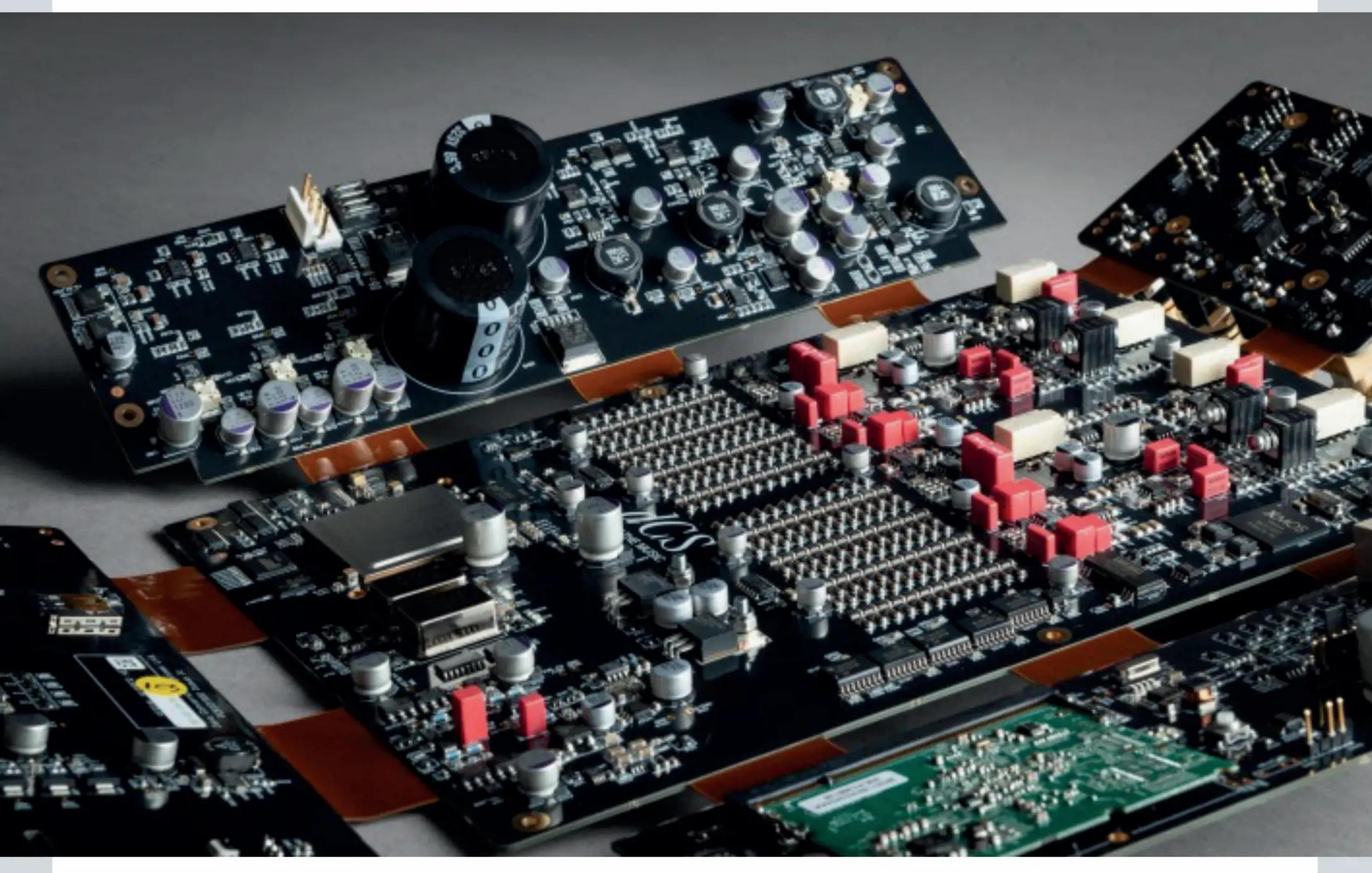
The four-way flex-rigid PCB found inside a Lina DAC X
