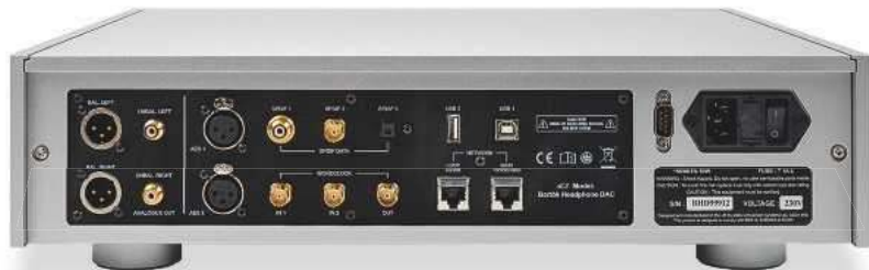
ABOVE: Digital inputs span S/PDIF (two coax, one opt), two AES/EBU (on XLRs), one USB-A for external HDDs, one USB-B for computer connection and a network loop (on RJ45s) – joined by clock I/Os (on BNCs) and variable analogue outs (RCA and XLR)
