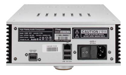
The rear view is uncluttered. There is no S/PDIF output, only USB.
