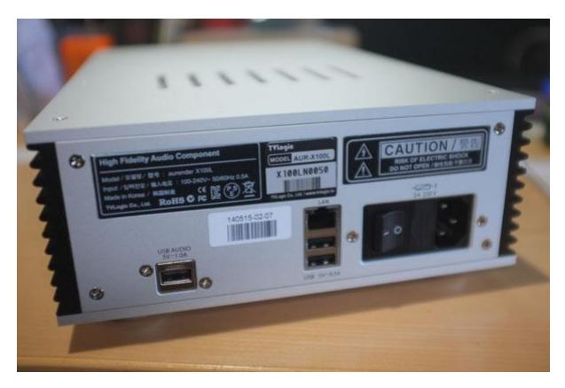
Inputs include Ethernet and 2x USB while outputs consist of a single USB socket to connect to your DAC. Aurender claims the lone USB output "is designed to deliver an exceptionally transparent audio signal free of noise and is shielded from outside electronic interference." Overall, I found the X100L to be exceptionally well made, concomitant with its price.
