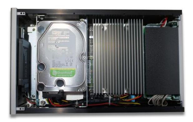
The hard drives are also physically isolated from the rest of the X100L's body to minimize their vibration and noise from traveling and infesting the audio signal. While you can see there is some care given to isolating the various functional parts, the X100L does not go to the same aluminum wrapped extremes as the S10.
