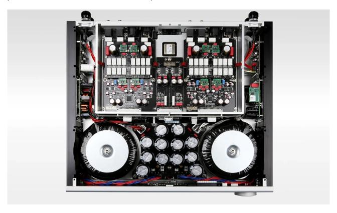
Now the AP20 story gets interesting. It's analog all the way from here on out (with one convenient exception). Aurender implemented an analog R2R stepped-attenuator volume control in the AP20. It would've been so simple for the company to just use the digital volume control built into the AKM chips, but I'm very happy an R2R analog control was selected because I often prefer the sound of a nice analog volume control.
