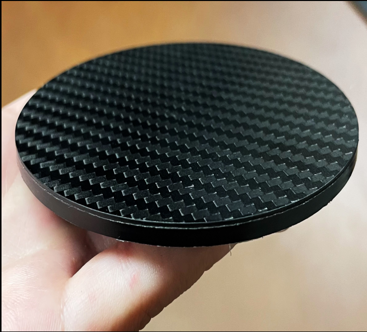
Moulded plastic that replicates carbon fibre
