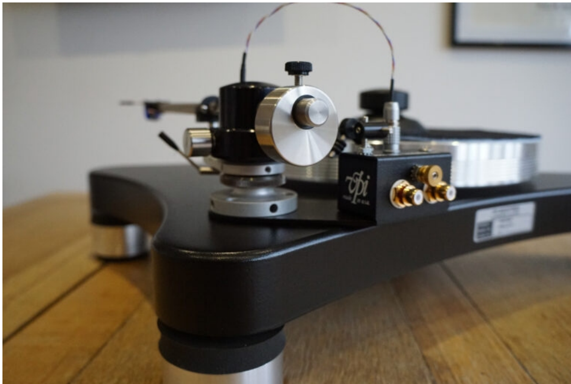
Armwire loop is used to generate anti-skate. Rear phono outputs are top quality and well spaced
