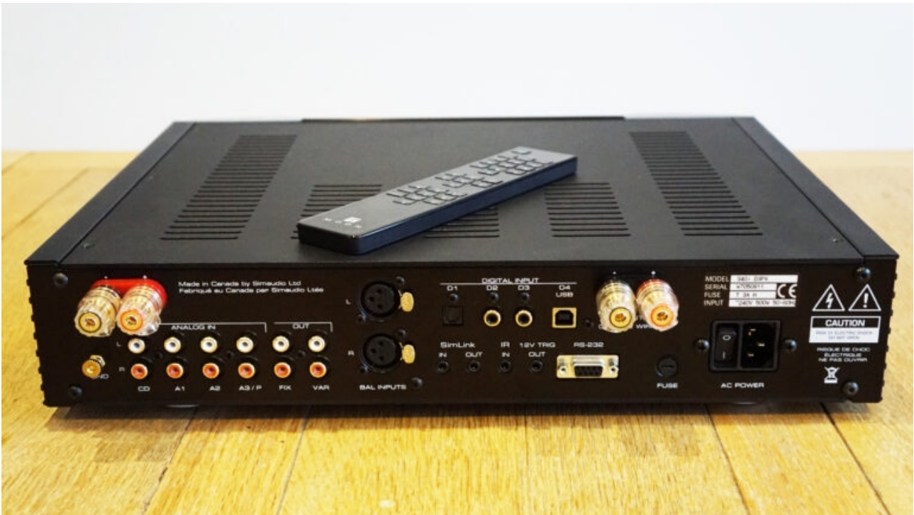
Five rear-panel analogue inputs include three line-level and one MM/MC over RCA, alongside a set of balanced XLRs plus fixed and variable outs. The D3 module adds S/PDIF over optical and coaxial, plus USB.
