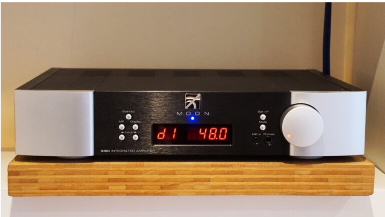
Front panel shows selected input alongside incoming sample rate. A 3.5mm input and 6.35mm headphone jack are handy add-ons
