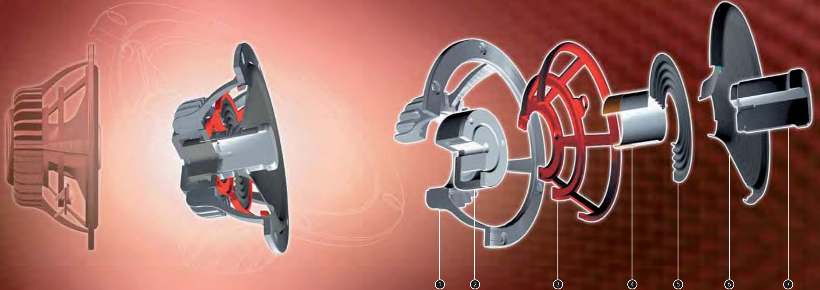
1. Aluminium diecast frame with integrated heat sink 2. Dual neodymium magnet system 3. Plastic inner basket optimised for high internal damping 4. 1 voice coil on black glass fiber bobbin 5. Conex spider 6. Ceramic coated aluminium cone with Active Cone Damping II 7. Solid, anodised aluminium phase plug
